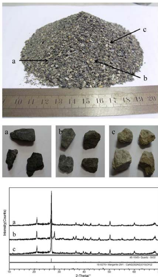
Fig. 5: Photograph and XRD patterns of CFBC bottom ash particles.
